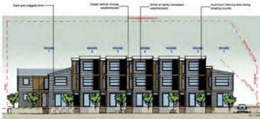
E-01 North-West Elevation (Street) Jan 2012
